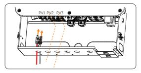
Figure 15-31 Connecting the PV cable
