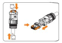
Figure 13-7 disconnector the AC connector
