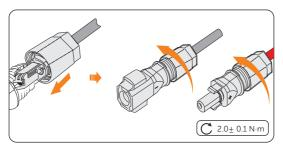
Figure 8-33 Tighten the cable gland
