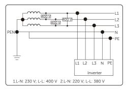
Figure 2-4 Supported power grid-TN-C-S
