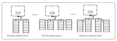
Figure 8-25 Battery connection Scheme 2
