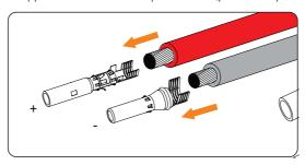
Figure 8-16 Inserting the PV pin contact
