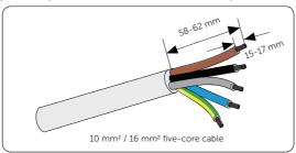
Figure 8-8 Stripping the Grid cable
