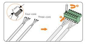
Figure 8-64 Connecting to 7-pin terminal block
