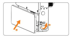
Figure 15-38 Installing the front panel
