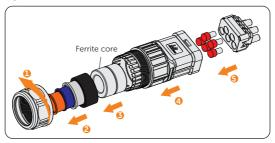
Figure 8-9 Disassembling the AC connector
