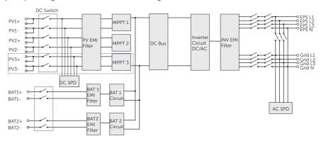
Figure 2-5 Circuit Diagram for X3-ULTRA series inverter
