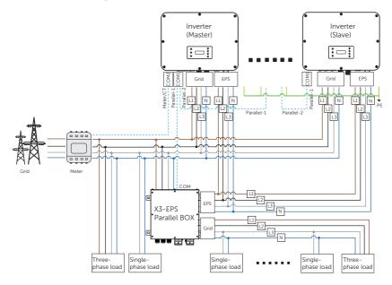
Figure 15-17 System diagram with SolaX X3-EPS Parallel BOX
