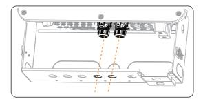
Figure 15-33 Connecting to COM terminal
