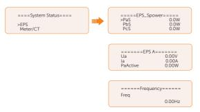
Meter/CT status: Information contains feed-in power of L1, L2 and L3 detected by the connected meter or CT. Positive represents feeding electricity to the grid, negative represents drawing electricity from the grid (buying electricity).
