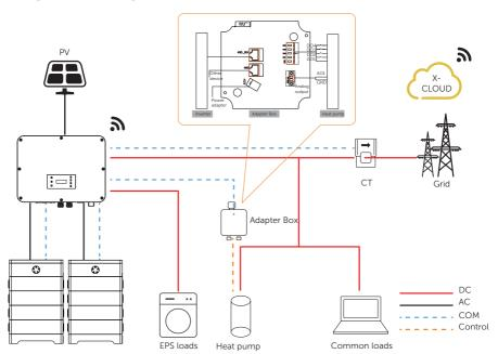
Figure 15-4 Adapter Box wiring diagram
