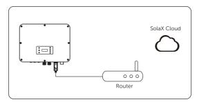
Figure 8-67 LAN mode connection diagram
