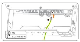
Figure 15-27 Connecting the PE cable
