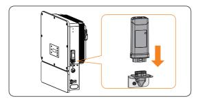
Figure 15-36 Installing the dongle
