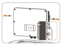
Figure 13-8 Unscrewing the M5 screws
