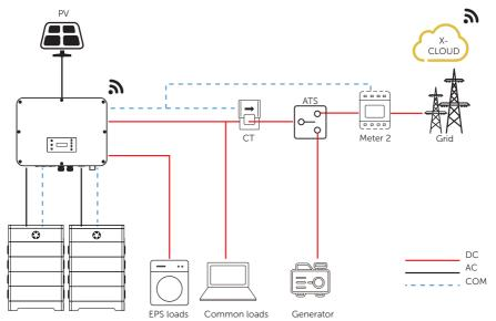
Figure 15-1 ATS control wiring diagram
