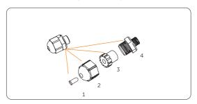
Figure 8-70 Disassembling the waterproof connector
