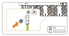
Figure 8-7 Securing the PE cable
