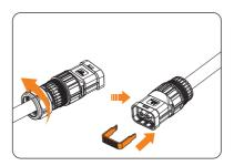
Figure 13-6 Remove the swivel nut
