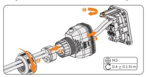
Figure 8-40 Securing the connector
