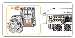
Figure 8-35 Removing the connector enclosure
