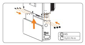
Figure 15-24 Installing the cable cover
