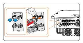
Figure 8-21 Connecting the PV cable
