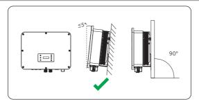
Figure 7-1 Correct installtion
