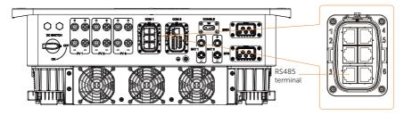
Figure 15-8 Connection terminal for EV-Charger
