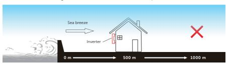
Figure 5-2 Incorrect installation position
