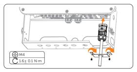
Figure 15-30 Installing the AC connector
