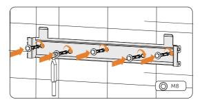
Figure 7-7 Inserting the screws
