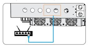
Figure 15-37 Installing the dongle
