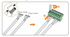
Figure 8-61 Connecting to 8-pin terminal block
