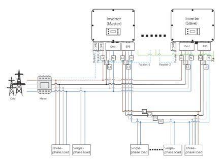
Figure 15-18 System diagram without SolaX X3-EPS Parallel BOX
