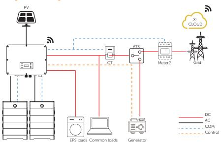
Figure 15-2 Dry contact wiring diagram
