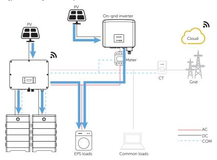
Figure 15-15 Power flowing when grid off
