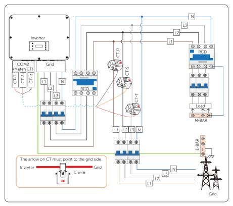
Figure 8-51 CT connection diagram
