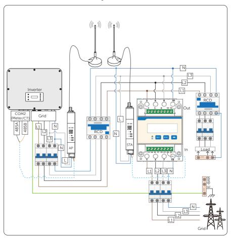
Figure 8-50 Wireless Meter connection diagram
