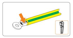
Figure 8-5 Crimping the cable
