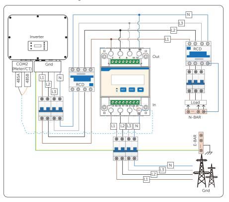
Figure 8-48 Meter connection diagram 1
