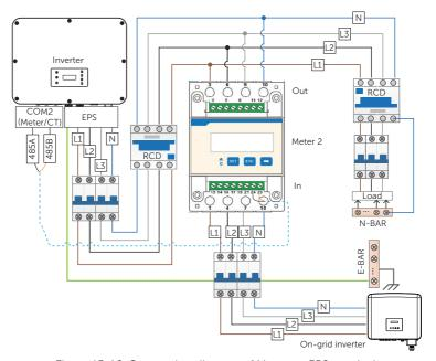
Figure 15-16 Connection diagram of Meter on EPS terminal
