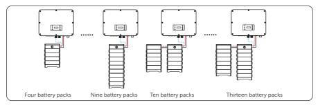
Figure 8-23 Battery connection Scheme 1
