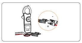
Figure 8-20 Measuring the voltage of PV connectors
