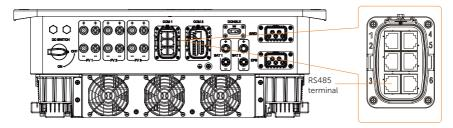
Figure 15-5 Connection terminal for Adapter Box
