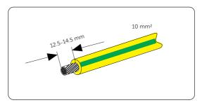
Figure 8-3 Striping the PE cable
