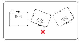
Figure 7-2 Incorrect installation
