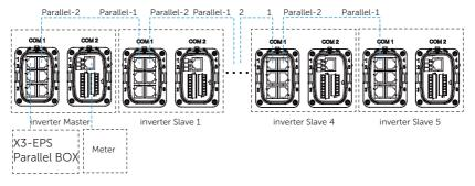
Figure 15-21 Communication connection with X3-EPS Parallel BOX
