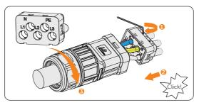
Figure 8-12 Assembling the AC connector
