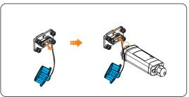
Figure 8-69 Wi-Fi connection procedure
