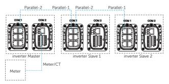
Figure 15-22 Communication connection without X3-EPS Parallel BOX
