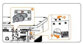
Figure 15-34 Installing the WiFi connecting cable
