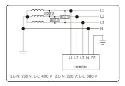
Figure 2-2 Supported power grid-TT
