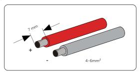
Figure 8-15 Striping the PV cable
