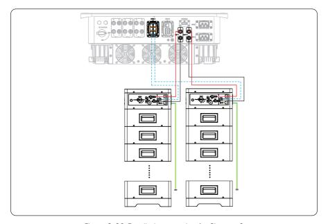
Figure 8-26 Detailed connection for Shceme 2
