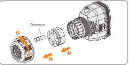
Figure 8-36 Disassembling the connector
