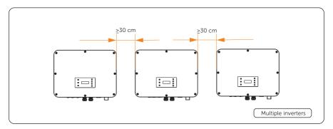
Figure 5-5 Clearance requirement for multiple inverter
