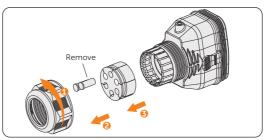
Figure 8-60 Disassembling the connector
