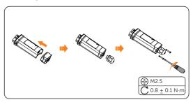
Figure 8-68 Assembling the dongle
