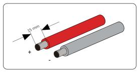
Figure 8-29 Striping the battery cable
