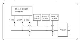
Figure 10-7 Phase Unbalanced enabled
