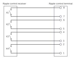
Figure 8-58 Connection diagram for ripple control
