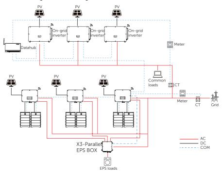
Figure 15-10 Datahub wiring diagram
