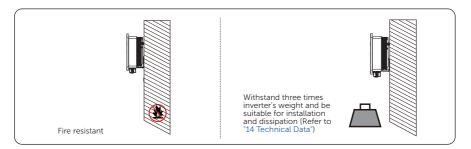
Figure 5-3 Installation carrier requirement
