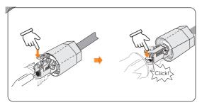
Figure 8-32 Press down on the Spring
