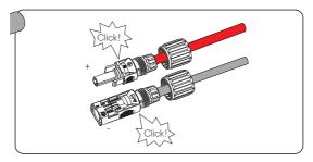
Figure 8-19 Securing the PV cable
