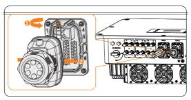
Figure 8-52 Disassembling the COM 2 terminal
