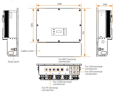
Figure 15-23 Appearance with cable cover (Unit: mm)
