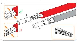
Figure 8-17 Crimping the terminal
