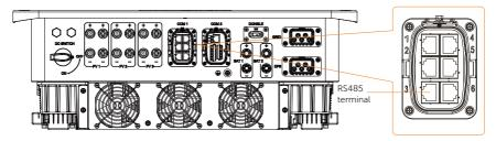
Figure 15-11 Connectiong terminal for Datahub
