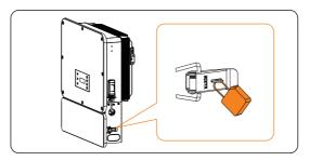
Figure 15-39 Installing the locks
