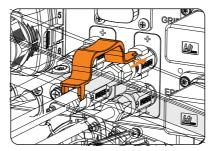
Figure 13-4 Removing the Battery connector
