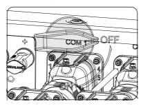
Figure 13-1 Turning off the DC switch
