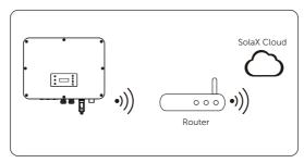
Figure 8-66 Wi-Fi mode connection diagram
