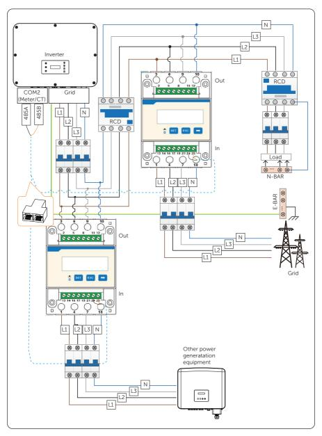
Figure 8-49 Meter connection diagram 2
