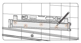
Figure 7-5 Marking the holes
