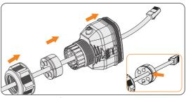
Figure 8-44 Threading the cables
