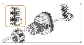
Figure 8-47 Installing RJ45 terminal to the cable fixture
