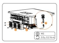
Figure 12-1 Disconnect the fans connectors
