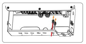
Figure 15-32 Connecting the battery power cable
