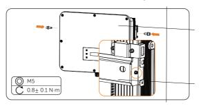
Figure 7-10 Securing the inverter
