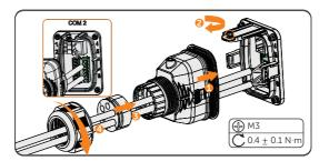
Figure 8-65 Connecting to the inverter
