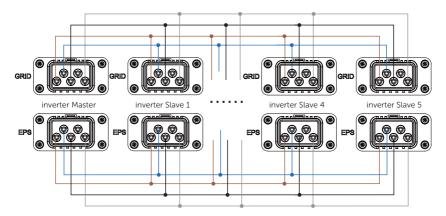
Figure 15-19 Power cable connection with X3-EPS Parallel BOX
