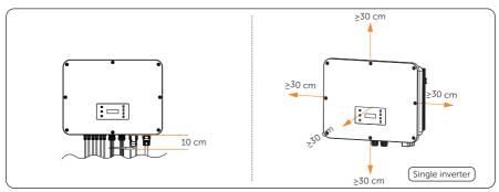
Figure 5-4 Clearance requirement for single inverter
