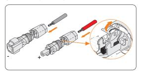
Figure 8-30 Opening the spring
