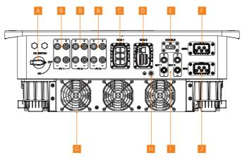
Figure 8-1 Terminals of Inverter
