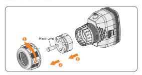
Figure 8-53 Disassembling the connector
