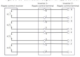
Figure 8-59 Connection diagram for ripple control in parallel
