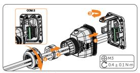
Figure 8-62 Connecting to the inverter
