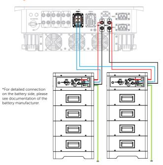
Figure 8-41 BMS connection diagram
