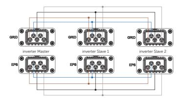
Figure 15-20 Power cable connection without X3-EPS Parallel BOX
