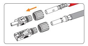
Figure 8-18 Threading the PV cable
