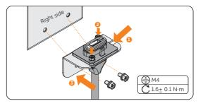
Figure 15-35 Installing the WiFi stand
