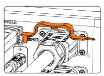
Figure 13-5 Removing AC connector
