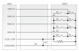
Figure 8-46 DRED wiring diagram
