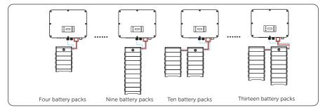
Figure 8-27 Battery connection Scheme 3
