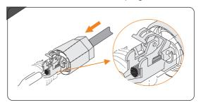
Figure 8-31 Threading the battery cable
