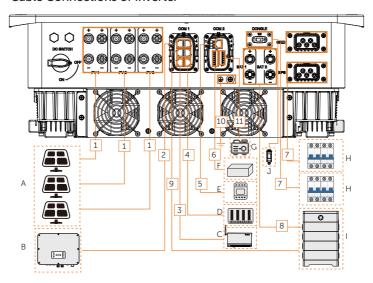
Figure 8-2 Cable connections of inverter
