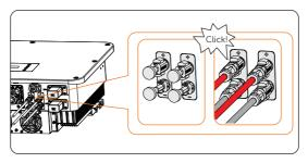
Figure 8-34 Connecting the battery connector
