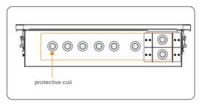
Figure 15-25 Removing the protective coil
