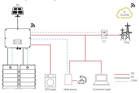
Figure 15-7 EV-Charger wiring diagram
