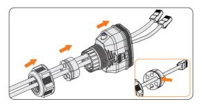
Figure 8-37 Threading the cables
