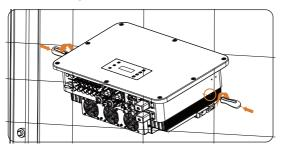
Figure 7-8 Installing the handles
