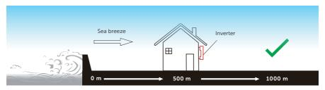
Figure 5-1 Recommended installation position
