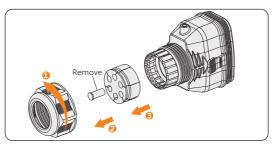
Figure 8-43 Disassembling the connector
