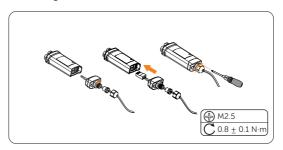
Figure 8-71 Assembling the dongle
