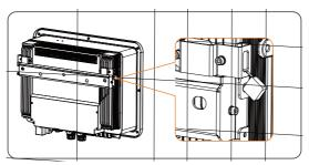
Figure 7-11 Locking the inverter
