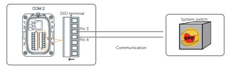
Figure 8-63 System switch connection diagram
