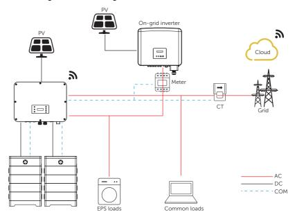
Figure 15-13 Micro-grid wiring connection
