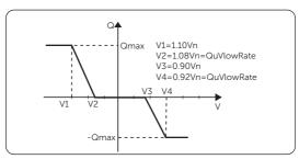
Figure 10-5 Curve Q = f(V))
