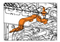
Figure 13-2 Releasing the PV connector
