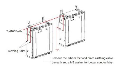
Step10. In order to remain the earth continuity on battery, Please following the procedure below for earthing.
