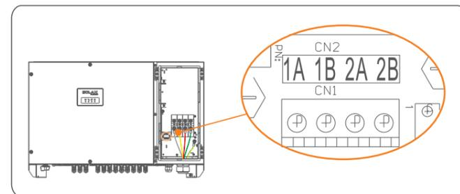
Interface of RS485 communications cable is in the right case of the inverter, shown in above figure.
