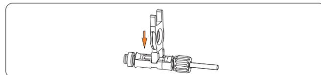
When uninstalling DC input connectors, insert removal wrench into the bayonet shown in Figure, press the wrench down, and take out the connector.
